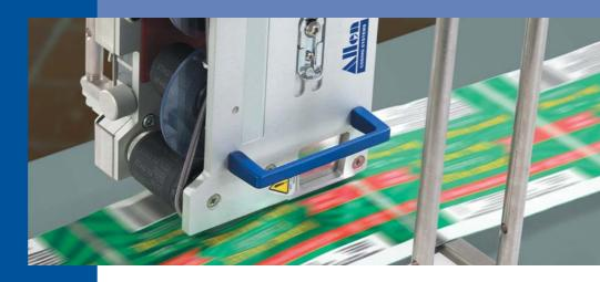
Online hot foil coders are used to code expiration dates, product identification information and lot/batch numbers onto labels and packaged products. With a vast range of frame designs, they are suitable for installation onto a wide range of packaging and labeling machines.
